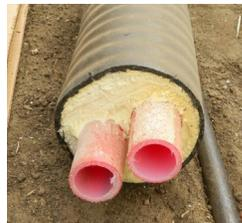
A less expensive underground insulated PEX tubing option (left) is wrapped in foiled bubble wrap and has space between the insulation on the pipe as well as the outer wall. Cost is approximately \$7.00/ft. The solid EPS insulated PEX tube (right) is more expensive at \$11.00/ft but has demonstrated reduced heat loss and pipe to pipe heat transfer. Water infiltration is a concern on the foil wrapped version on the left due to the open area that exists.
