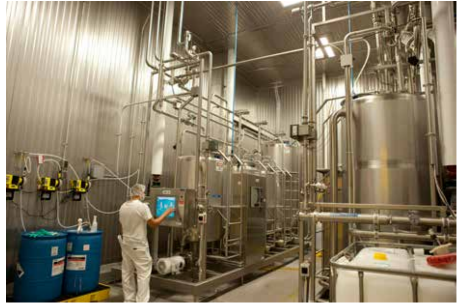
Commonwealth's Clean In Place (CIP) process.
