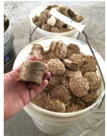
Fuel "pucks" or "briquettes" made from Switchgrass by Renewable Energy Resources for combustion testing.
